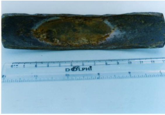
Fig. 1 black deposits & Brown oxide film on the inner surface
